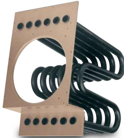
One standard feature of all Lennox unit heaters and duct furnaces is the tubular heat exchanger, designed to enhance performance and reliability. The exchanger's curved design provides excellent heat transfer by completely exposing the heating surface to the air stream. Rounded surfaces minimize air resistance and even heating is allowed across all surfaces, reducing stress on the heat exchanger.
